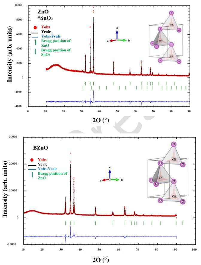
The good agreement between experimental and fitting diffraction lines ensures the hexagonal structure of ZnO and BZnO samples with a Space group P63mc and there are no signs of a
