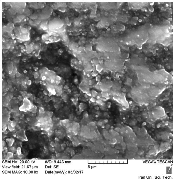
Fig.3. the microstructure of nitrated pellet at 1573°k
