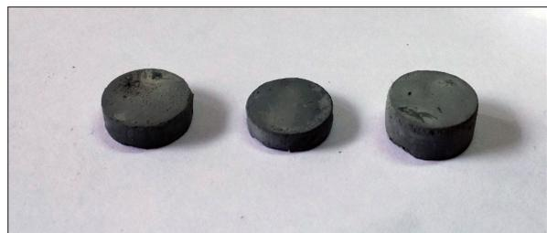
Fig.2. compacted pure silicon after pressing
